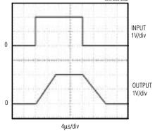
$V_{CC} = \pm 2.5V$   $R_L = 1k\Omega$ ,  $C_L = 15pF$  $A_V = 1V/V$
